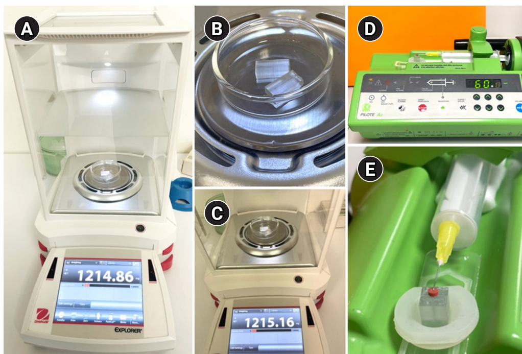
Figure 2. (A–C) High-precision microbalance (Explorer Semi-Micro; Ohaus Corporation, Parsippany, NJ, USA) used to weigh samples at different experimental stages. (D, E) Syringe pump (Pilote A2; Fresenius Vial SAS, Brézins, France) used for controlled delivery of sodium hypochlorite during the experiments.
