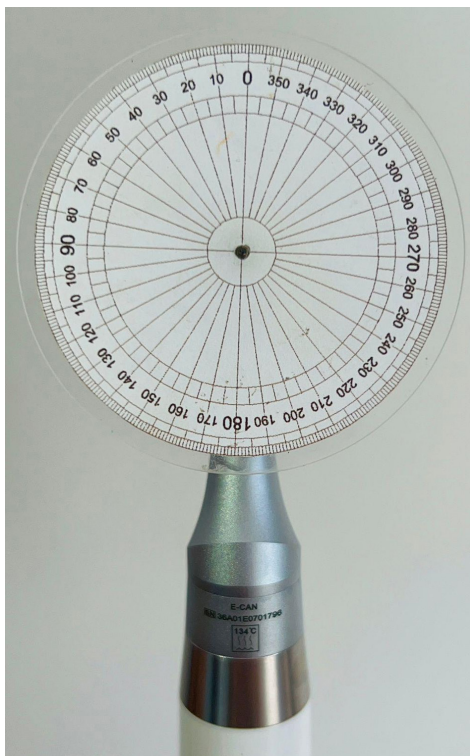
Figure 1. A 5-cm-diameter polypropylene disc marked in degree intervals from 0° to 360° was used in the experiment.
